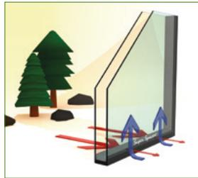
In the summer Super Spacer® minimises the heat exchange at the edges of the window panes and keeps the cool air indoors.
