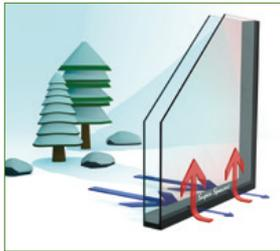
In the winter Super Spacer® ensures even temperature distribution at the window pane and keeps the heat in the building.
